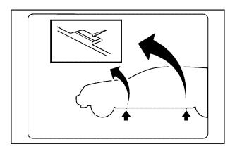
Find the jacking location using the diagram above and corresponding V-shaped locating notches located in the plastic molding.
